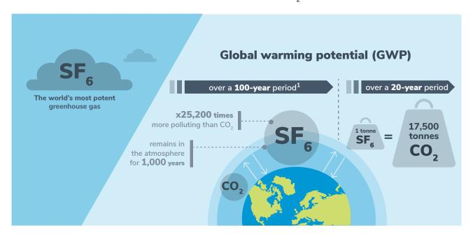
Despite its potency, the use of  ${\rm SF_6}$  continues increasing virtually unabated. Emissions from leakages occur during the installation, maintenance, dismantling, replacement, and operation of electrical switchgear, circuit breakers and transformers.
